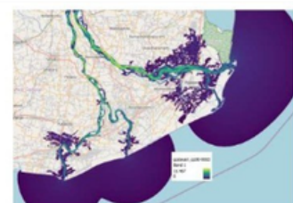
Figure 3. Godavari basin — simulated maximum inundation extent, Q100 design flood.
